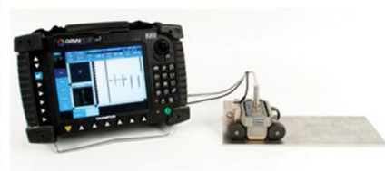
Calibration over reference material and specific EDM notches.
