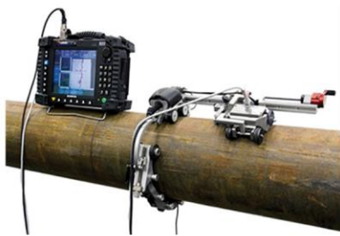
Eddy Current Array Semi automated Solution for Pipeline Surface Cracking Inspection.
