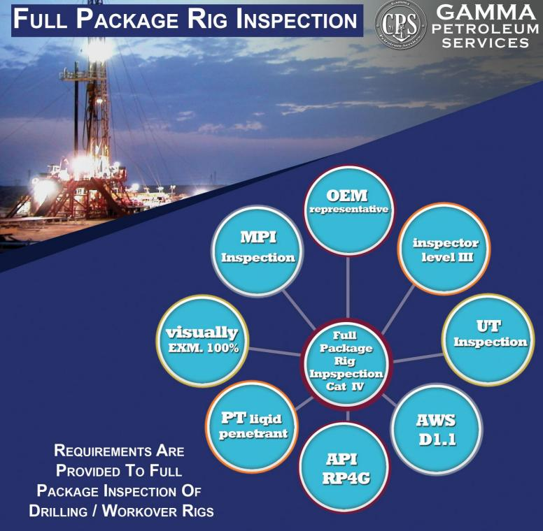
Category IV - Category IV includes Category III requirements but adds disassembly, inspection, and cleaning required to conduct NDT of all defined critical areas. All welds are being visually examined and welds in critical areas should be inspected using magnetic particle or liquid penetrant method in accordance with Section 6 of AWS D1.1.
